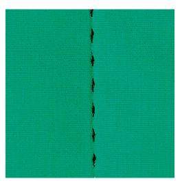
Handlook quilt stitches are suitable for all fabrics and sewing projects which should look hand sewn. It is recommended to use a monofilament thread as upper thread and an embroidery thread as bobbin thread. The sewing speed should be moderate to prevent the monofilament from breaking. If required, the upper thread tension and the balance can be adjusted to the sewing project and the desired quilt stitch.
