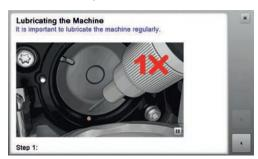
> Give one drop of oil in each of the two oil depots so that the felts are damp and make sure that the redmarked surface of the hook sleeve remains free of oil.
