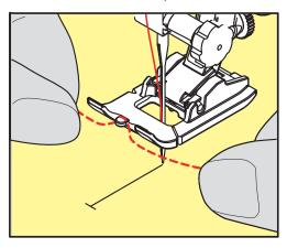
> Pull both cord ends under the buttonhole foot to the back and insert each a cord into the slits of the sole.
