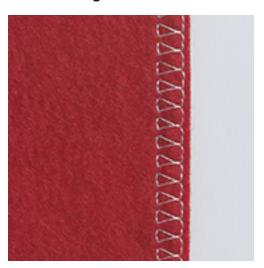
A double overlock seam is suitable for loose knitware and cross seams in knits. When working with knitware, a new jersey needle should be used to prevent damaging the delicate stitches. When sewing elastic materials, use a stretch needle.
