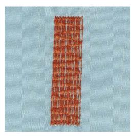
The reinforced Darning Program No. 23 is especially suitable for quick darning of worn or damaged areas. The reinforced Darning Program No. 23 replaces threads along the lengthwise grain in all materials.
