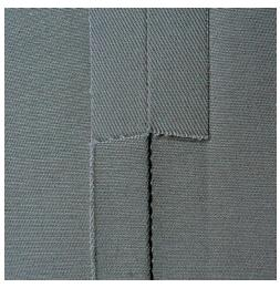
The Triple Straight stitch is especially suitable for durable seams and for firm, densely woven fabrics such as denim and corduroy. For firm or densely woven materials it is recommended to attach the Jeans foot No. 8. This will help to sew denim or canvas. For decorative topstitching the stitch length can be elongated.
