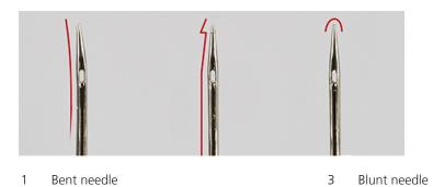
2 Damaged needle point
